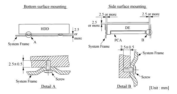
Figure 4.3 Mounting frame structure
